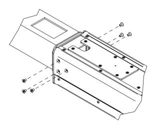
7. Lift the VIDA M using a suitable lift and slide it onto the stand with the Universal Header HD attached.
