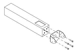
4. Slide the mounting-plate tabs into the corresponding inlets of the speaker.
